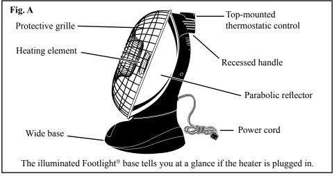
ON. In addition, the buzzer may sound and the heater will shut off if too much dust or dirt has accumulated on the parabolic reflector. To clean the parabolic reflector, see cleaning instructions on page 4.
